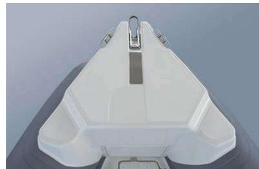
**A large bow nose** with two side bollards and a stainless steel anchor housing is designed for the installation of an electric windlass.
