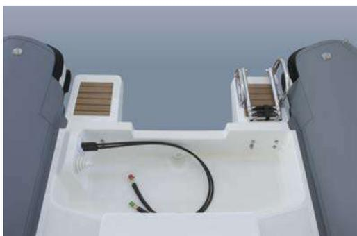
The hull of the Coaster 650 is much appreciated for its tightness and softness that make it a flexible boat for both fun and work. Pleasant to maneuver even with impervious sea and with engines ranging from 100HP (minimum) to 200HP. The extreme stern allows you to install **two additional fiberglass panels** with teak inserts and is equipped with lifting hooks installed on the transom. A small locker provides additional storage space for ropes and fenders.
