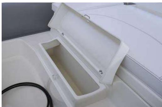
**The extreme stern** has a compartment suitable for stowage of mooring lines or of the stern anchor.
