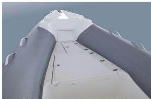
Below are **two peaks** that exploit the full depth of the hull, one for stowage of the anchor and chain and the other for various materials.
