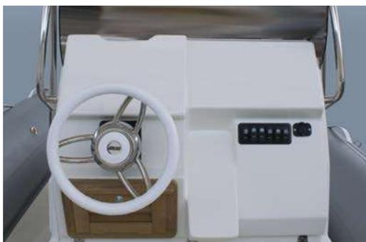
As in all Coaster, **the console is positioned laterally** on the right side of the boat but with a central guide, leaves ample space on the left side allowing a wider and easier passage from stern to bow. The console is designed to allow the installation of one or more screens.
