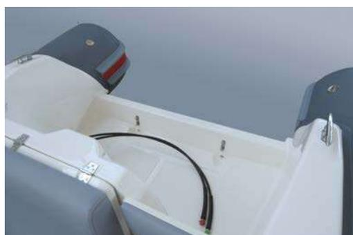
**The transom and bilge cockpit** are accessible through an entrance in the lateral part of the stern wall. The ascent space from the aft ladder is wide enough to access easily. Two side cleats for mooring lines and aft eyebolts are installed on the transom for lifting the boat. Two extra fiberglass platforms can be installed on the transom to enlarge the boat further.
