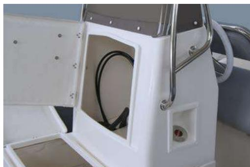
**The console** has two inspection hatches for convenient and quick access in case of maintenance of the on-board instruments.
