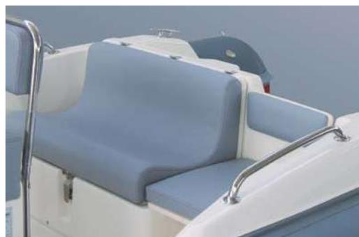
The **stern cockpit** has a comfortable shape for navigation thanks to the three-seat dinette which is divided into two fixed parts and one mobile. The fixed part can accommodate two people and is equipped with a locker underneath for stowage of various materials. The removable part of the dinette instead, consists of a side extension to allow a third person to sit down.
