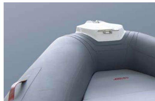
At the far bow a **fiberglass nose** with stainless steel cleats for fixing the mooring lines provides also an anti-slip platform for ascending/descending. **Handles** on the tubes guarantee greater safety during navigation.
