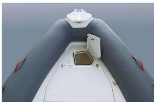
Underneath the pillows of the bow sunbathing area, **two lockers**: one for the anchor and one for general storage, characterise the deck.
