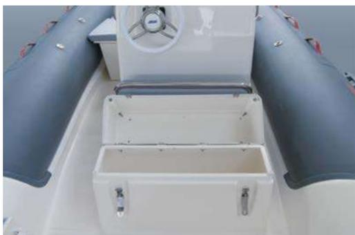
The seat opens towards the console, providing an additional storage area.
