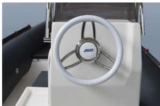
**The console** positioned laterally on the starboard side of the boat but with a central driving, leaves ample space on the port side allowing a wider and easier passage from stern towards the bow. Despite being small in size the console area has sufficient space for the installation of basic navigation instruments. The height of the console is optimal for standing and seated riding.
