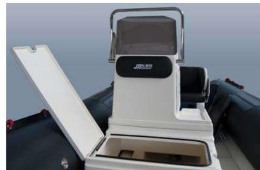
Under the seat, **a locker** gives to access the console. Inside this locker lies the fuel tank, concealed under a wooden floor. This floor creates a surface divided from the fuel tank to allow placement of objects in the console.
