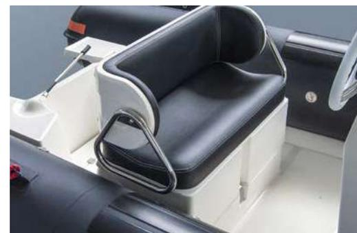
**The aft seat** consists of a comfortable cushion suitable for two people to sit. Equipped with a rotating backrest, it allows the captain to use it as a back rest while standing up. At the stern beneath the driving seat a **large and deep locker** characterises the aft storage space.
