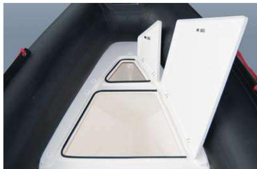
Under the bow sundeck, **two comfortable lockers** compose the available storage space. The first was designed for the anchor and the chain while the second for stowage of various materials or for safety equipment.
