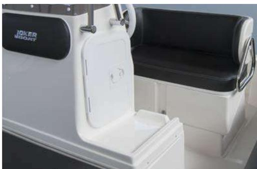
On the side of the console a **useful inspection hatch** allows a quick intervention in case of need whilst an integrated shelf provides extra storing space. **The windshield**, with stainless steel handrail, protects the pilot and provides an extra grip for the safety of passengers during navigation.
